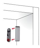
3 ANTI-TURNOVER LOCKING Stop screwing the red bolt when it touches the wall plate
